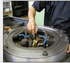
ground pieces are then thread rolled
