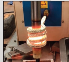
The trimmed slugs are induction heated.
