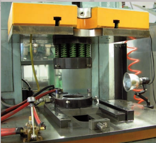
110 Ton OBI Hot Forging Press Equipped with Adjustable Slide Table and Custom Base Plate
