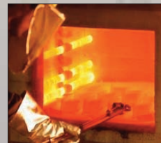
Headed blanks are heat-treated,
